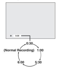
When the unit reaches the specified time, it will be turned off automatically.
